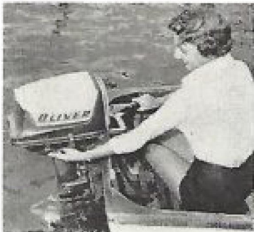
The Oliver 6's ease of servicing is demonstrated here as this young skipper releases the hood-catch, allowing her to remove the entire motor hood.
